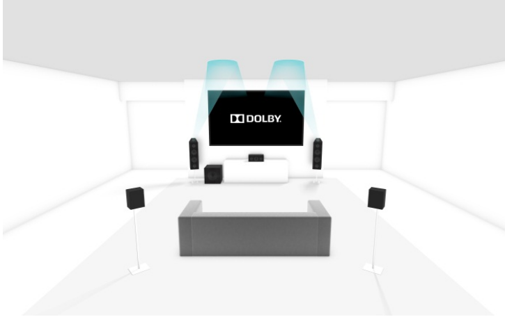
Figure 7: A traditional 5.1 speaker layout with two Dolby Atmos enabled speakers (5.1.2).
