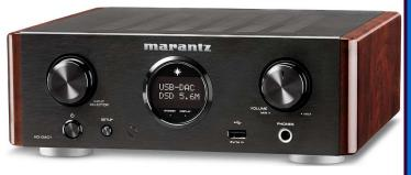
The amp can push multiple headphone impedance levels, including the big 600 ohm guys, and feed your powered stereo speakers sweet sound as well. It can even be a great DAC for your computer - via it's built in USB-B connection.
